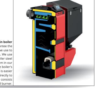
Applied technology in boiler manufacturing. We guarantee the quality of the materials we use to manufacture our products. We use only attested, high-grade boiler steel with a thickness of 6 mm in our boilers. Thanks to the boiler's three-section design, it is easier to install and transport directly to the boiler room. The boiler consists of a body, fuel dispenser and burner.
