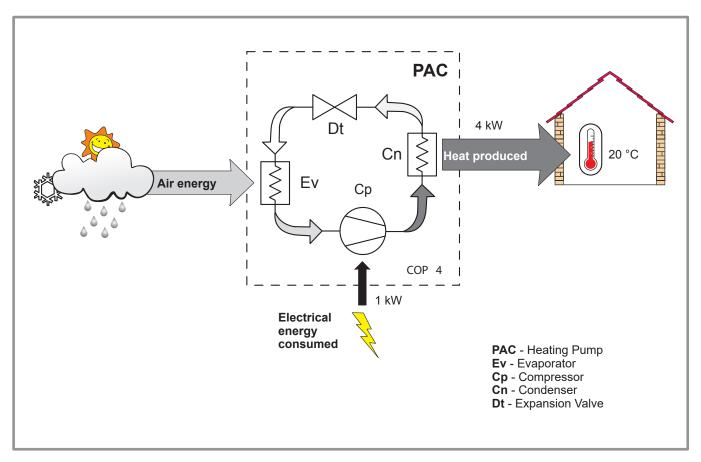
figure 11 - Heat pump operating principle
