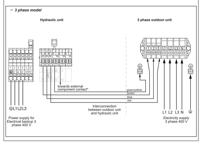
figure 37 - Connection to terminal blocks and power relay
