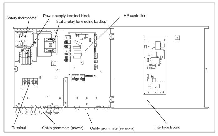
figure 39 - Description of the 3 phase hydraulic unit's electrical control box
