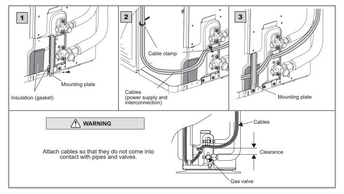
figure 32 - Finalising connection of single phase outdoor unit
