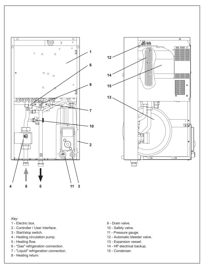
figure 9 - Hydraulic unit components
