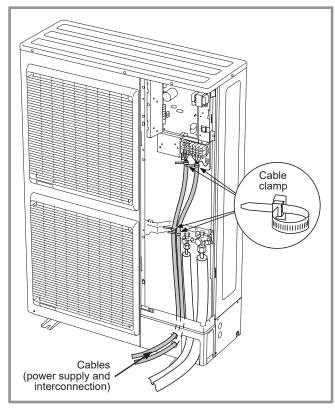
figure 35 - Finalising connection of 3 phase outdoor unit
