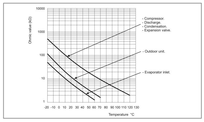
figure 7 - Ohmic sensor values (Outdoor unit)
