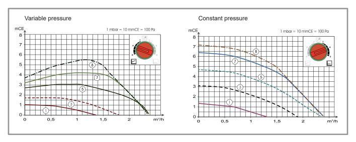
figure 6 - Available hydraulic pressures and flow rates
