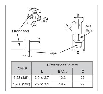
figure 17 - Flaring of the flared connections
