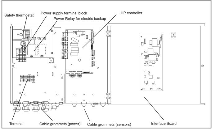
figure 38 - Description of the single phase hydraulic unit's electrical control box
