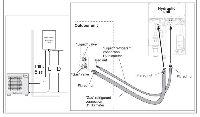
figure 19 - Refrigeration connections (authorised diameters and lengths)
