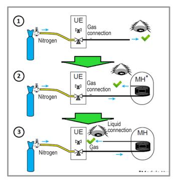
figure 21 - Checking refrigeration connections
