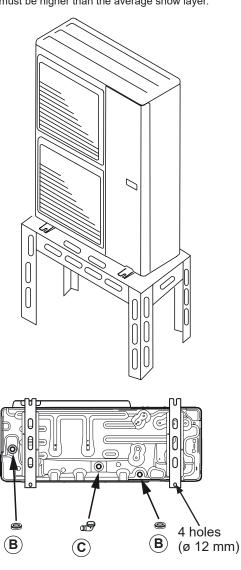
figure 14 - Installation of the outdoor unit evacuation of condensates
