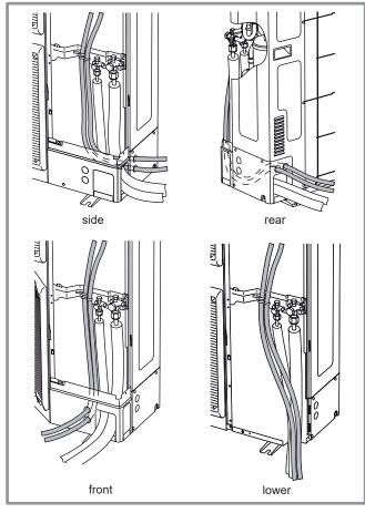
figure 36 - Feeding cables and refrigeration connections from the 3 phase outdoor unit
