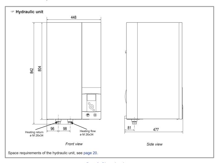
figure 2 - Dimensions in mm
