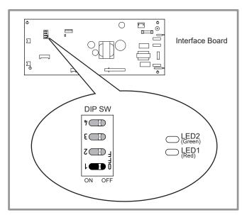
figure 24 - Location of DIP switches and LEDs on the hydraulic unit interface board
