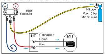
If a pressure drop occurs, bring it back down to 1 bar and look for leaks with a leak detector, repair and repeat the test.
