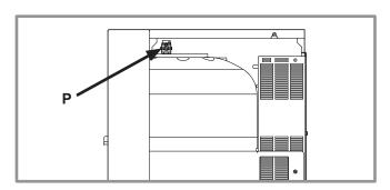
figure 25 - Hydraulic unit automatic bleeder valve
