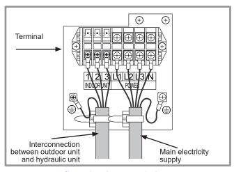
figure 34 - Access to 3 phase outdoor unit's terminal block
