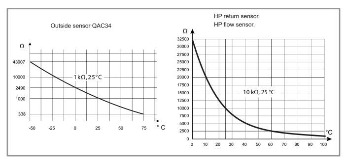
figure 5 - Ohmic sensor values (Hydraulic unit)
