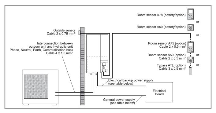
figure 29 - Overall layout of electrical connections for a simple installation (1 heating circuit)
