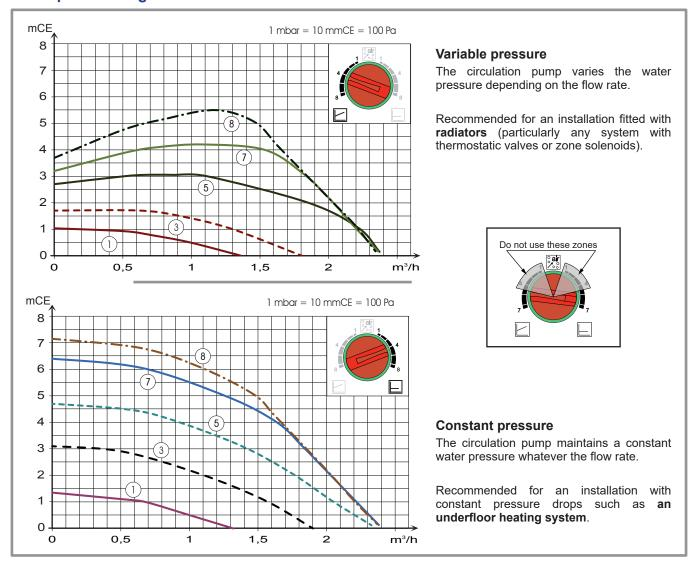
figure 26 - Available hydraulic pressures and flow rates
