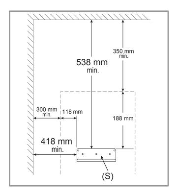
figure 15 - Mounting bracket
