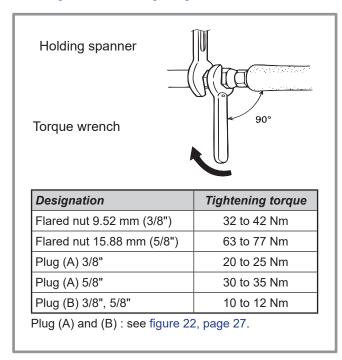
figure 20 - Tightening torques
