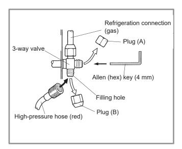
figure 22 - Connecting the hose to the gas valve
