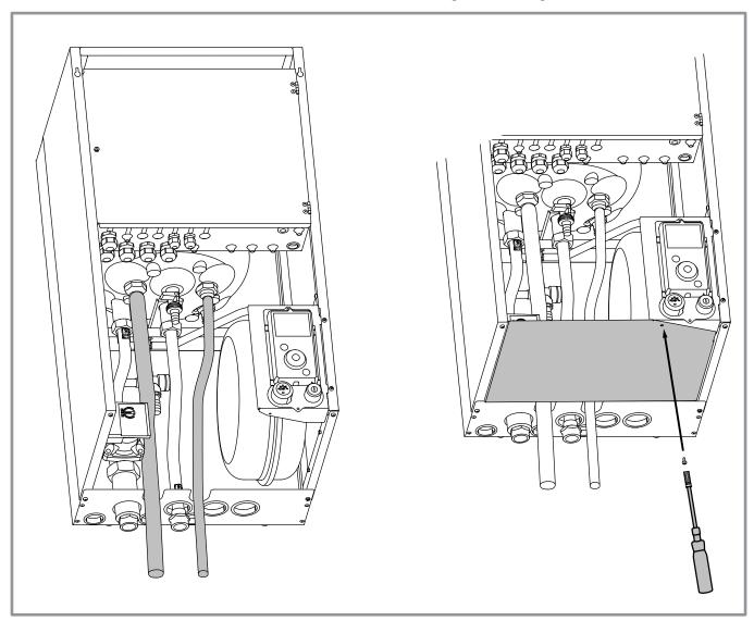
figure 18 - Feeding through flared connections
