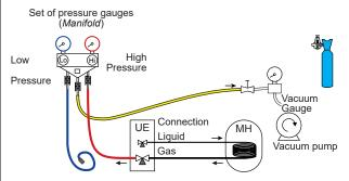
**b**) Switch off the vacuum pump, close the valve at the end of the service hose (yellow), connect this hose to the expansion valve on the nitrogen bottle, fill to 2 bar, close the hose's valve again,
