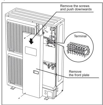
figure 33 - Access to 3 phase outdoor unit's terminal block
