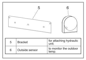
figure 4 - Accessories provided with the hydraulic unit
