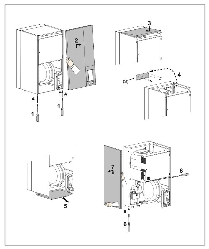
figure 16 - Removing the casing
